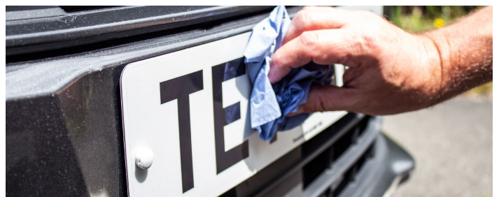
6. Polish plate using circular motion with a soft cloth to remove finger prints.
