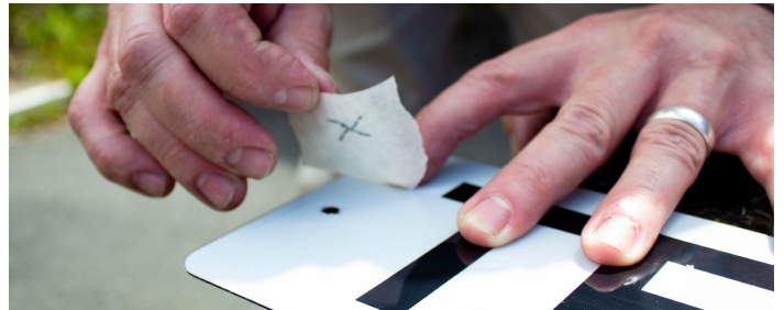
4. Remove masking tape and de-burr holes.
