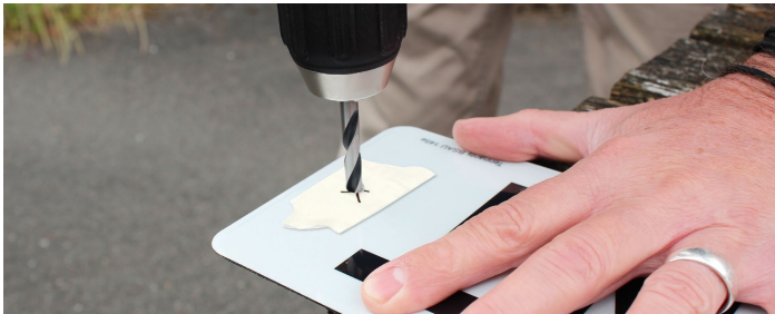
3. Using a 6mm diameter acrylic bit, drill from the FRONT of plate. (Allow drill to do the work - don't apply too much pressure).
