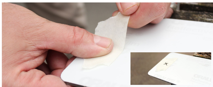
2. Apply a small piece of masking tape where hole is to be drilled.
