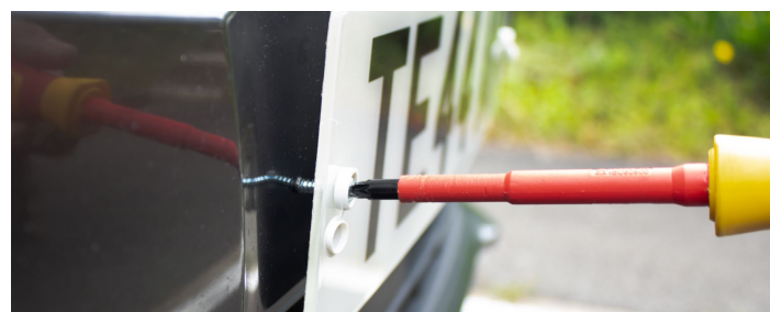
5. Position plate in correct location and carefully tighten fixings.
